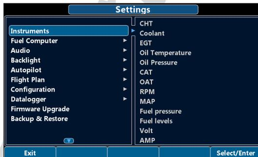
The labels near the button indicate their function within the menu. Use the knob to scroll between items then push the button to select it. If the highlighted item is a submenu, in the right side of the screens, a preview of its items is visible.
