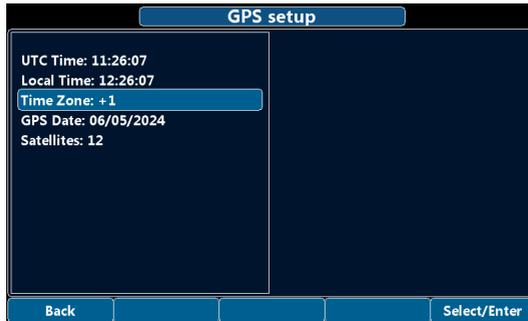
This page can be used to verify the correct functionality of the GPS. In case of incorrect baud rate, or no communication on the serial port, the time information (date and time) will not be displayed.
