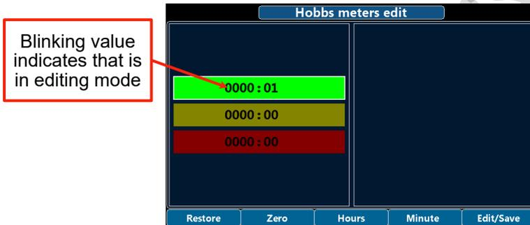
1. Rotate the knob to select the desired range to edit then press the knob button to confirm.
