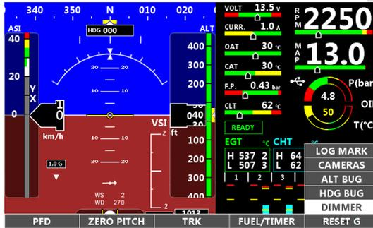
The labels near the button indicate their function within the menu. Use the knob to scroll between items in the right list, then push the button to select it. For example if DIMMER is selected the popup menu will change as in the picture below.
