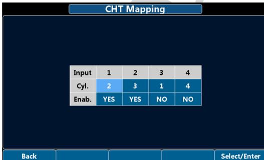
Although we recommend to perform a clean installation, with this feature it's possible to reassign or disable the different CHT inputs: for example you can assign the *Input #1* to the engine *Cylinder #3* and so on. You can also disable each inputs, useful for example if a sensor fails and you don't want to display the indication for that sensor.
