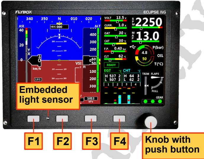
Pushbuttons are used to switch between different screens and perform different action within them. When inside a menu, or a popup menu is visible, the meaning of the pushbuttons is always indicated.
