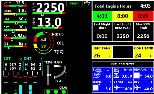
EIS (*Engine Information System*) working mode is used to monitoring only engine data. All available indications are the same of the IFIS mode (right side).
