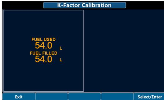
7. In the FUEL FILLED field, now insert the exact quantity of fuel you have added and measured in step #4; probably it doesn't correspond exactly to the FUEL USED because this is the measurement from the transducer not yet calibrated and it's showed for reference only. To insert the value rotate the knob then press on *Enter* to calculate the new value.
