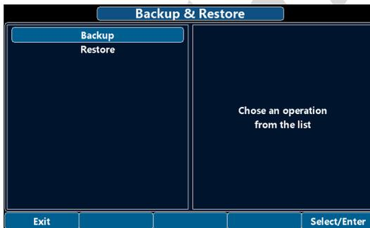
**Backup:** insert a USB flash drive in the USB rear connector on the *Eclipse NG* and then press *Enter* with this item selected to save all the settings on the USB 2.0 flash drive. The file is *ECLIPSE\_NG\_<ID>.par* (where ID is the unique ID of the device).
