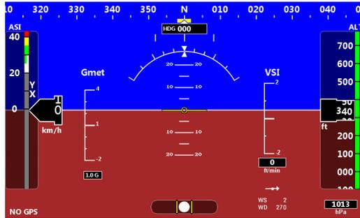
PFD (*Primary Flight Display*) working mode is used to monitoring only flight data. All available indications are the same of the IFIS mode (left side).
