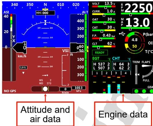
IFIS (*Integrated Flight Information System*) working mode divide the display in two areas of monitoring. On the left side are present all attitude and air data, allowing monitoring of flight parameters. Available indication are:
